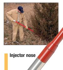
Spring-loaded injector head
