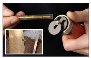
Simply load shells into lance end, screw on end cap, and begin injecting. Lance shaft contains four chambers into which shells are loaded. Fully loaded, the lance weighs less than ten pounds.
